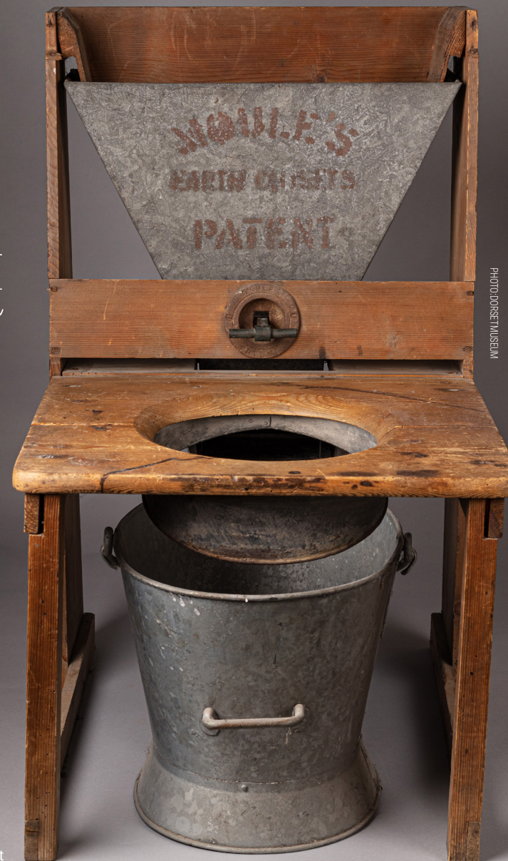
Henry Moule's 1873 patented earth closet
