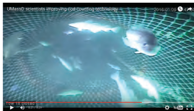
The new video system uses a mounted camera to capture images of fish passing through an open-ended fishing net. Researchers then review the video to count the different species, and estimate the size of each fish.
