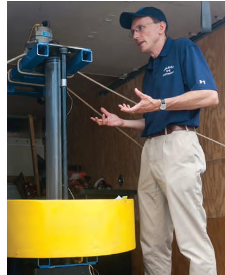
Dr. MacDonald's low-cost WEC device captures small amounts of ocean wave energy as two objects move against each other.
