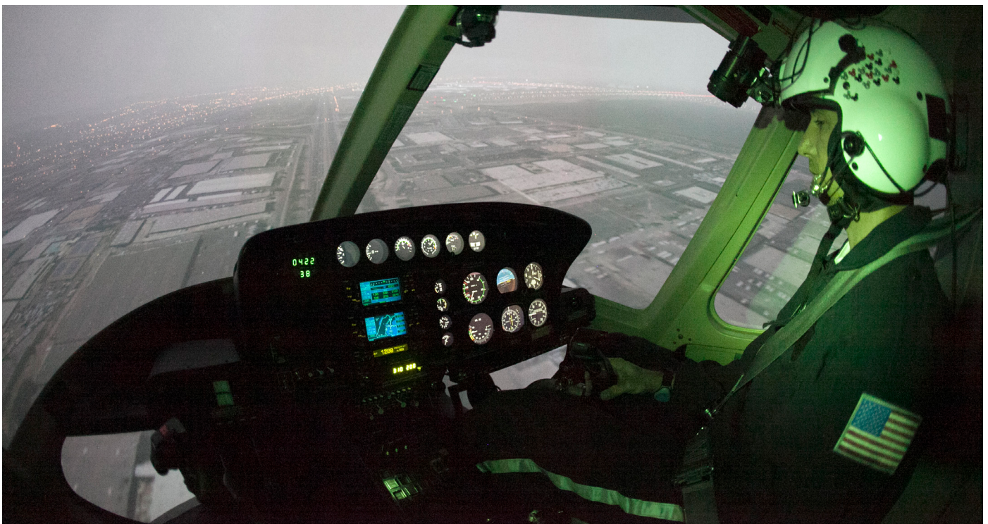
Specialty training such as night-vision goggle or inadvertent entry into instrument meteorological conditions can be accomplished in a certified FFS or FTD, regardless of aircraft model.
