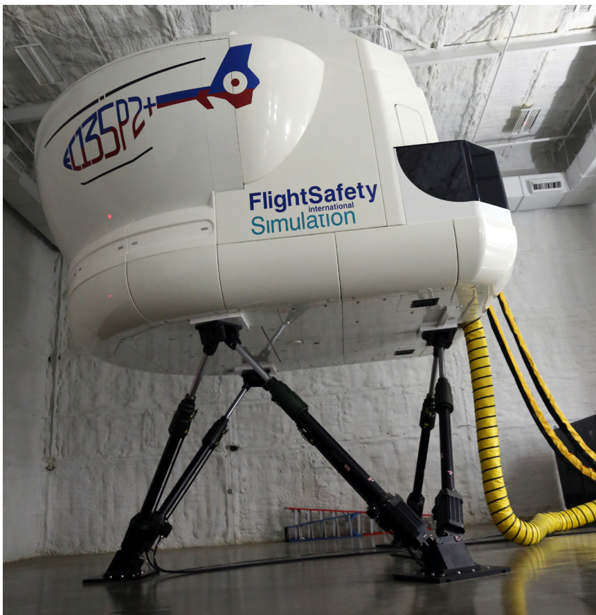
The realism of the training environment provided by this FFS Level D simulator for an EC135 P2 aircraft is enhanced by motion, visual, and sound cues.
