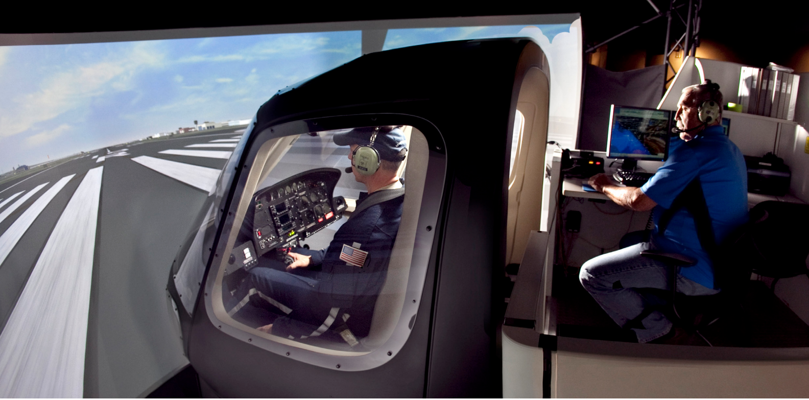
Using the same visual graphics as an FFS, this Level 7 FTD provides a realistic flight environment for pilots. The instructor at the right can program location and weather conditions and system malfunctions.
